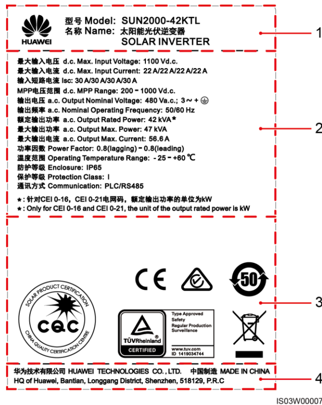
Figure 2-9 Nameplate of the SUN2000-42KTL
