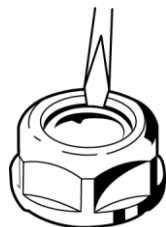
Figure 5-7 Stripping a seal ring
